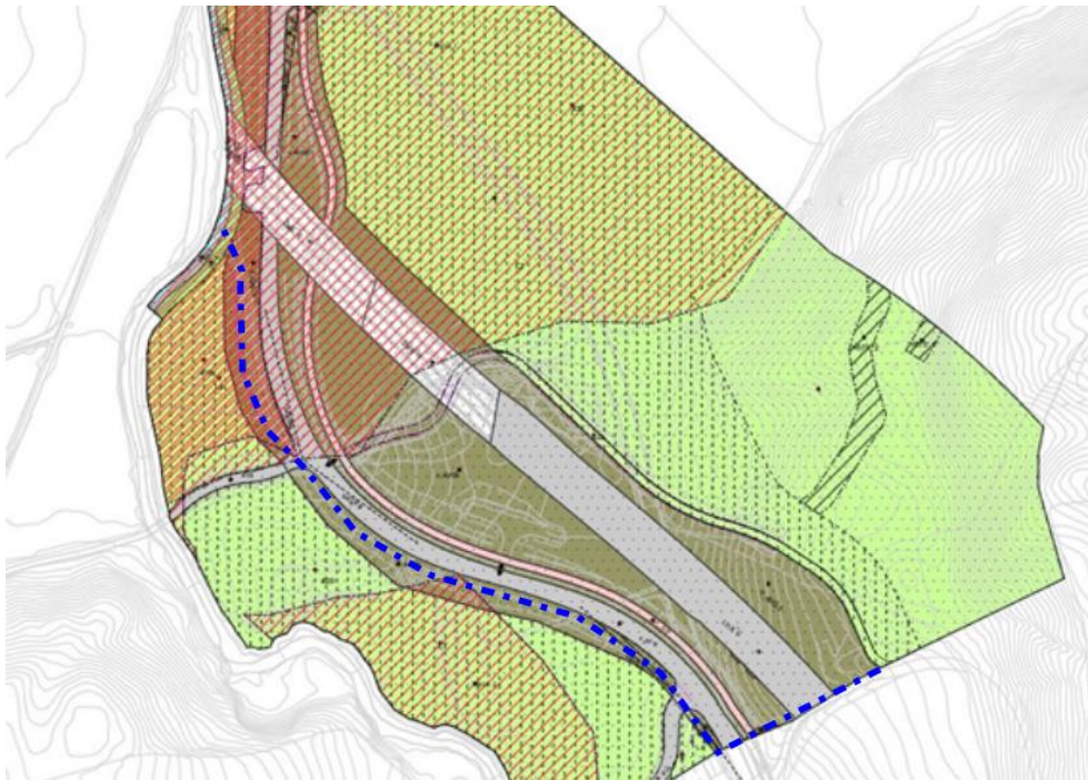
Figur 9 Trase for overvann
