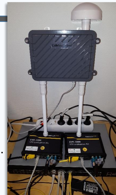
Picture shows two car radios from Kapsch and one infrastructure radio from Cohda Wireless
